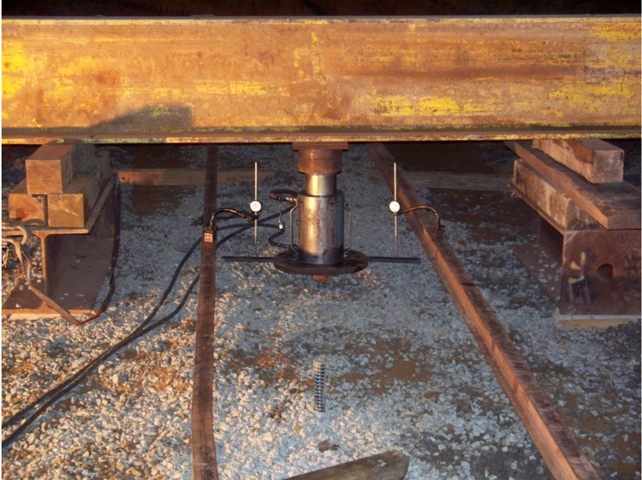
Figure 9 - Proof Load Testing Apparatus
